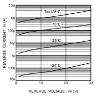
Fig. 2 Reverse characteristics
