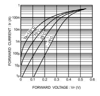
Fig. 1 Forward characteristics
