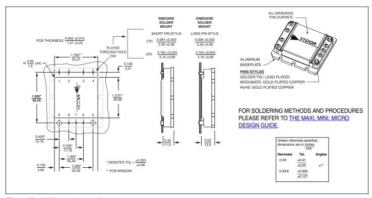
*Figure 13*—*PCB mounting specifications*
