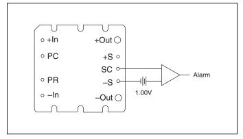
Figure 7 — Secondary side on-state indicator.
