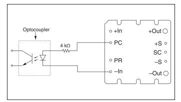
Figure 6 — Isolated on-state indicator.
