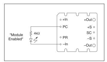
Figure 4 — LED on-state indicator.
