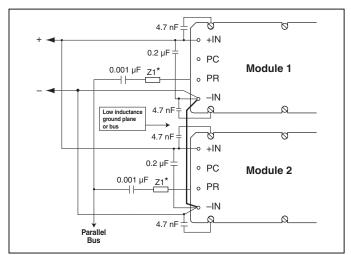
*Figure 9* — *AC coupled single-wire interface.*
