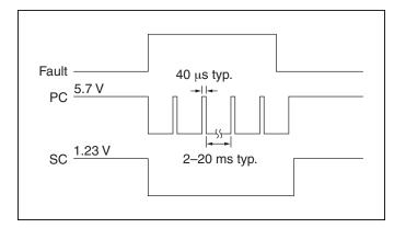
*Figure 5* — *PC/SC module alarm timing.*
