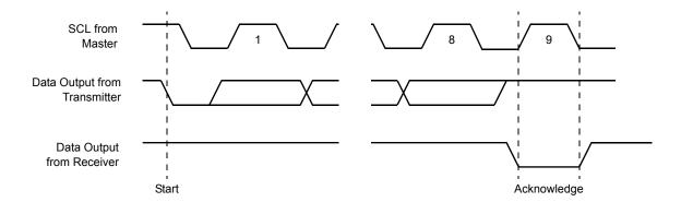
Figure 10. Byte Write Sequence
