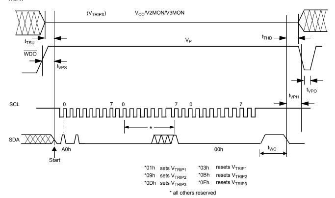
V<sub>TRIP1</sub>, V<sub>TRIP2</sub>, V<sub>TRIP3</sub> Programming Specifications: V<sub>CC</sub> = 2.0 - 5.5V; Temperature = 25°C
