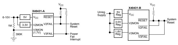
Notice: No external components required to monitor three voltages.
