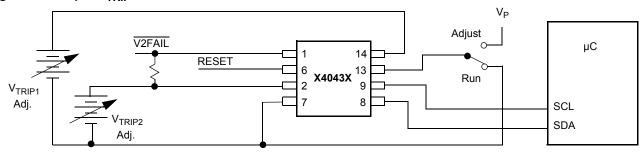
Figure 6. V<sub>TRIPX</sub> Set/Reset Sequence (X = 1, 2, 3)
