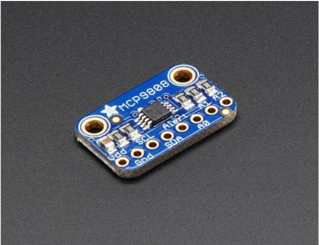
This I2C digital temperature sensor is one of the more accurate/precise we've ever seen, with a typical accuracy of ±0.25°C over the sensor's -40°C to +125°C range and precision of +0.0625°C. They work great with any microcontroller using standard i2c. There are 3 address pins so you can connect up to 8 to a single I2C bus without address collisions. Best of all, a wide voltage range makes is usable with 2.7V to 5.5V logic!
