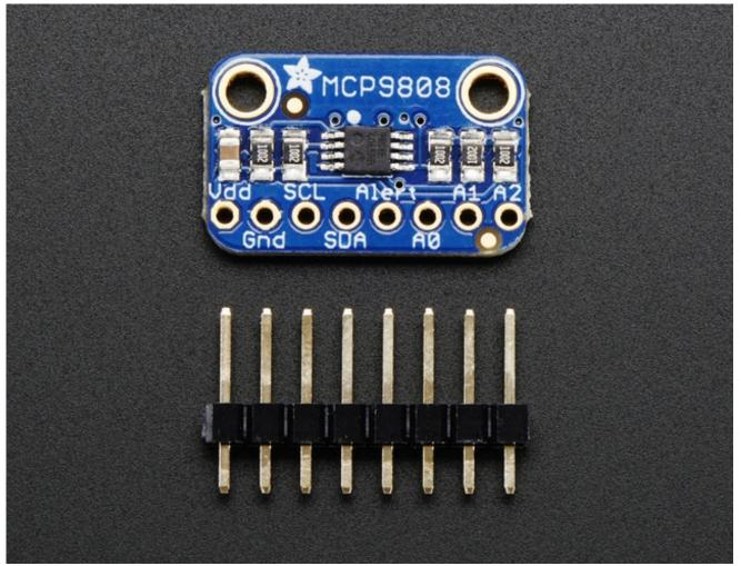
Unlike the DS18B20, this sensor does not come in through-hole package so we placed this small sensor on a breakout board PCB for easy use. The PCB includes mounting holes, and pull down resistors for the 3 address pins. We even wrote a lovely little library for Arduino that will work with any Arduino compatible. You'll be up and running in 15 minutes or less.
