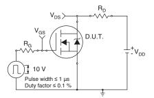
Fig. 10a - Switching Time Test Circuit
