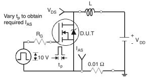
Fig. 12a - Unclamped Inductive Test Circuit
