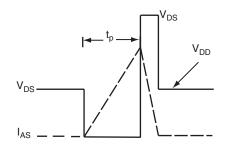
Fig. 12b - Unclamped Inductive Waveforms
