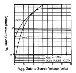
Fig. 3 - Typical Transfer Characteristics
