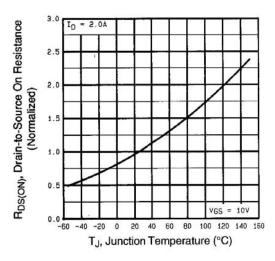
Fig. 4 - Normalized On-Resistance vs. Temperature
