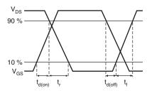
Fig. 10b - Switching Time Waveforms
