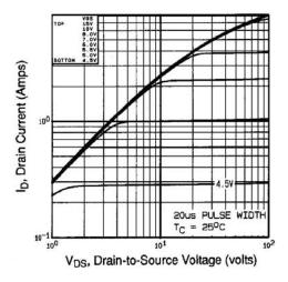
Fig. 1 - Typical Output Characteristics,  $T_C = 25$  °C
