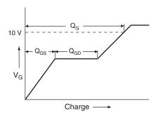
Fig. 13a - Basic Gate Charge Waveform
