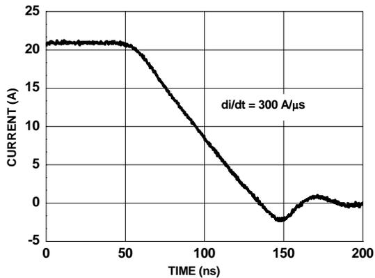
Figure 14. FDMS0309AS SyncFET<sup>™</sup> body diode reverse recovery characteristic
