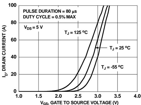
Figure 5. Transfer Characteristics
