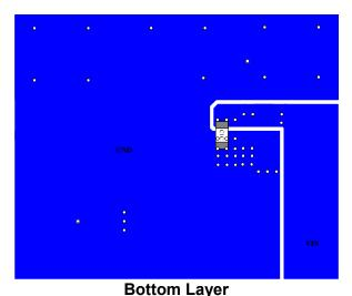
Figure 14: 13-Pin QFN MP8763 PCB Layout Guide
