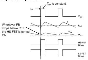
Figure 2: Heavy-Load Operation
