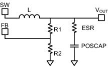
Figure 10: Simplified POSCAP Circuit
