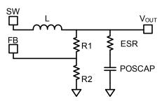
Figure 6: Simplified PWM-Mode Circuit without External Ramp Compensation
