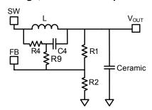
Figure 11: Simplified Ceramic Capacitor Circuit
