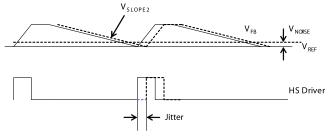
Figure 5: Skip-Mode Jitter Ramp with a Large ESR Capacitor
