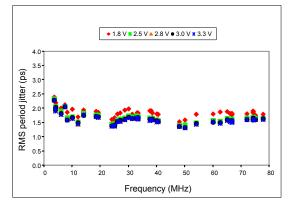
Figure 8. RMS Period Jitter vs Frequency
