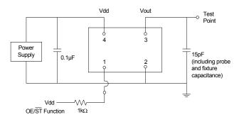
**Figure 1. Test Circuit**
