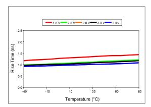
Figure 12. Rise Time vs Temperature, 20 MHz Output
