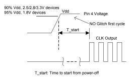
Figure 3. Startup Timing (OE/ST Mode)
