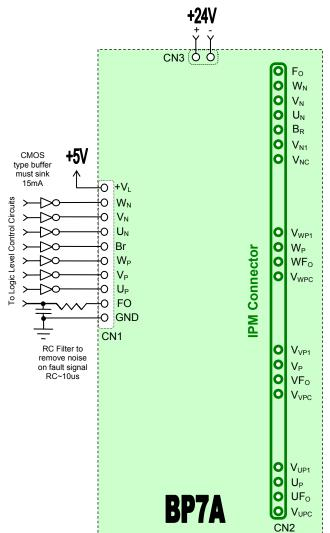
Figure 4: BP7A External Connections
