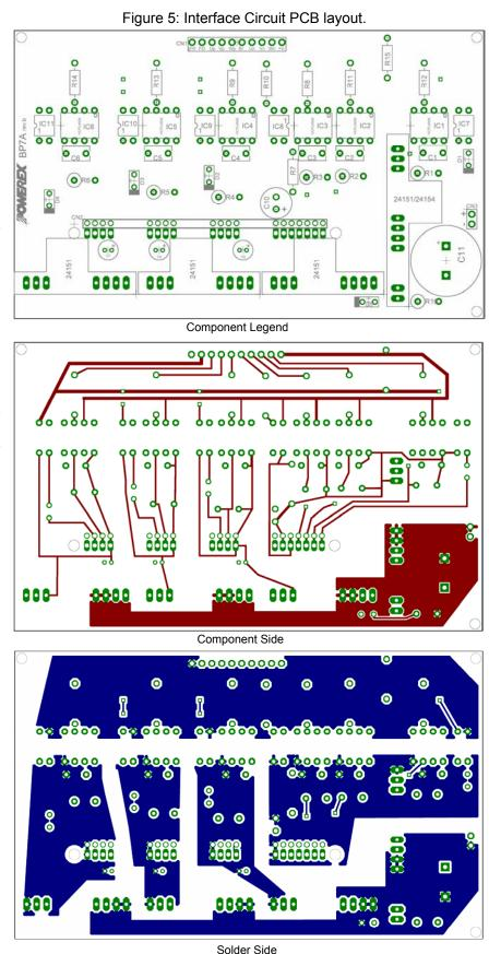
the current limiting resistors (R9-R14) must be adjusted. The value of the limiting resistor can be calculated by assuming the forward voltage drop of the optocoupler's photodiode is approximately 1.5V and that the buffer/driver on-state output voltage is approximately 0.6V. For example, if a 15V logic power supply is desired, the required limiting resistors would be: (15V-1.5V-0.6V)÷16mA = 800Ω.
