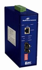
This quick installation guide describes how to install and use the hardened compact Media Converter. Capable of operating at temperature extremes of -40 to +75°C, this is the media converter of choice for harsh environments constrained by space.
