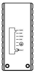
While only one power source is required to power up the media converter, two power sources offer redundancy for those mission critical applications. (PWR1 and PWR2)
