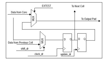
Figure 25.4 Diagram of Output Cell
