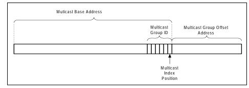
Figure 17.2 Multicast Group Address Region Determination
