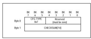
Figure 12.8 Configuration Done Sequence Format
