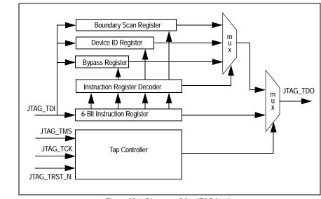
Figure 25.1 Diagram of the JTAG Logic
