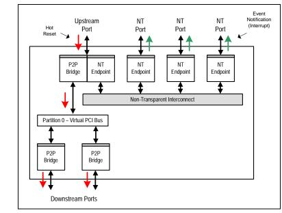
Figure 1.16 Example of Switch Event Mechanism
