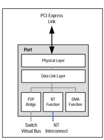
Figure 1.2 Logical Representation of a Port with PCI-to-PCI bridge, NT, and DMA Functions
