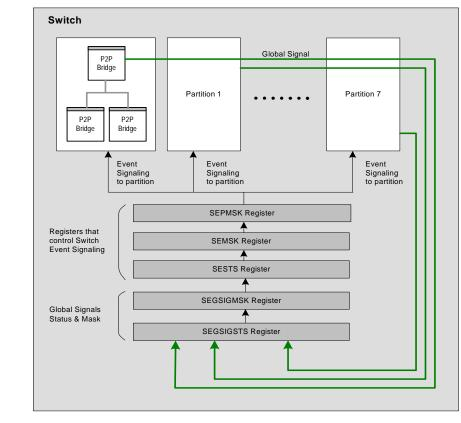
Figure 16.2 Global Signaling Mechanism
