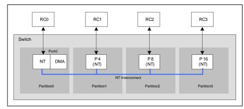
Figure 26.19 PES32NT8xG2 with Port 0 Configured in NT Function with DMA Mode and Ports 4, 8, and 16 in NT Function Mode
