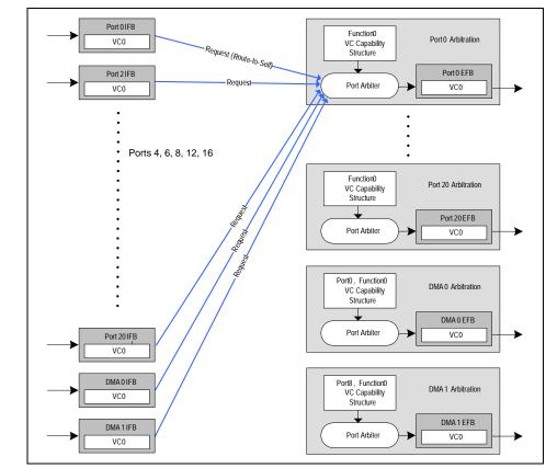
Figure 4.2 Architectural Model of Arbitration
