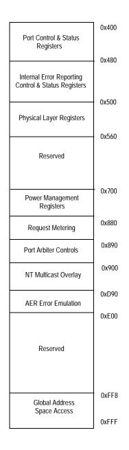
Figure 19.2 Proprietary Port Specific Register Organization
