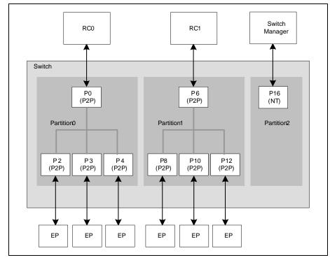
Figure 26.5 I/O Load Balancing Example: Initial Switch Configuration
