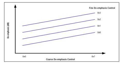
Figure 8.1 Relationship Between Coarse and Fine De-emphasis Controls
