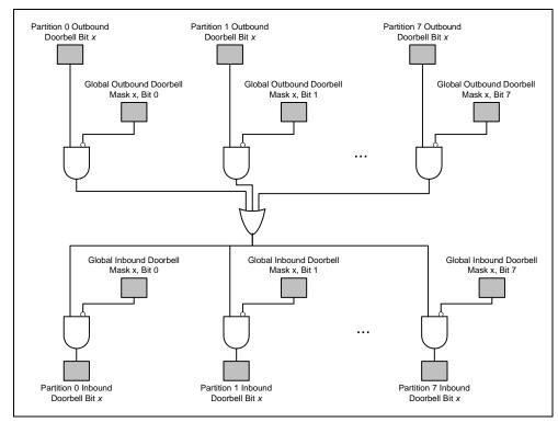
Figure 14.9 Logical Representation of Doorbell Operation
