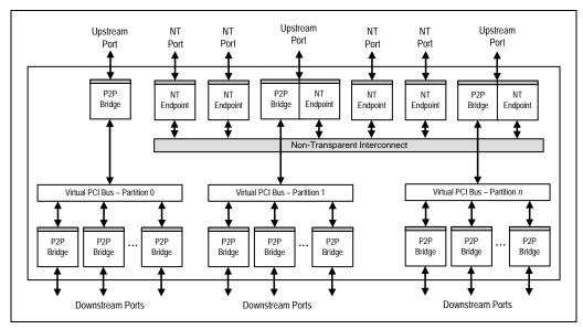
Figure 1.11 Non-Transparent Switch with Non-Transparent Ports
