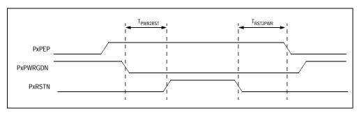
Figure 11.5 Power Good Controlled Reset Output Mode Operation
