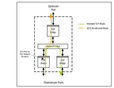
Figure 10.3 ACS Peer-to-Peer Request Re-direct at a Downstream Switch Port
