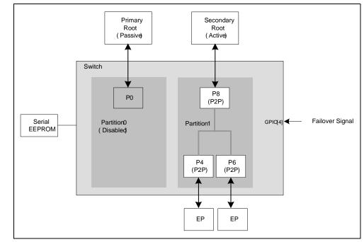
Figure 26.13 Active/Passive System Configuration after Failover Event
