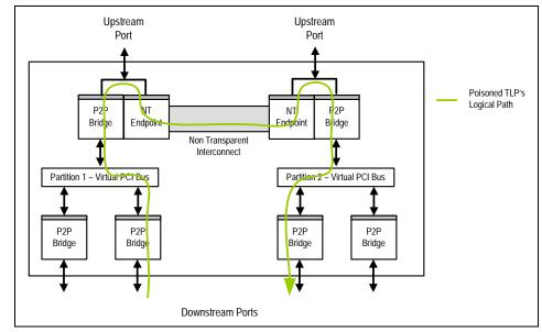
Figure 14.16 Poisoned TLP Error Propagation Example
