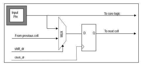
Figure 25.3 Diagram of Observe-only Input Cell
