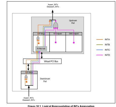
Figure 10.1 Logical Representation of INTx Aggregation
