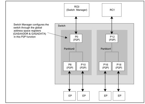
Figure 26.4 PES16NT8BG2 with Two Partitions Configured via a Switch Manager Root Complex
