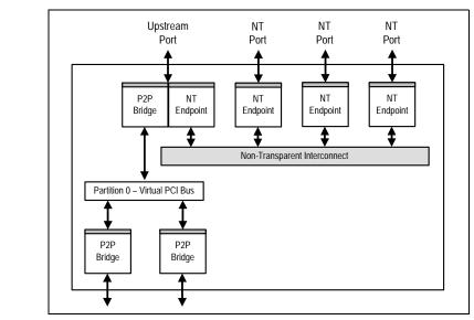
Figure 1.9 Non-Transparent Switch with Non-Transparent Ports
