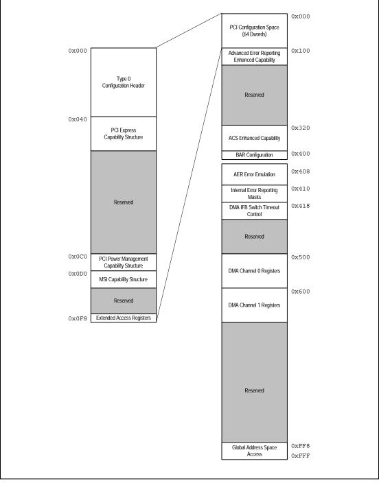
Figure 19.4 DMA Function Configuration Space Organization
