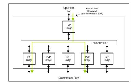
Figure 1.17 Example of Transparent Multicast
