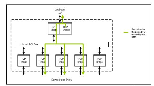
Figure 15.12 Path Taken by a TLP Emitted by the DMA When it is Multicasted<sup>1</sup>
