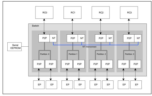
Figure 26.7 Multiprocessor System Interconnection Using the PES32NT8xG2
