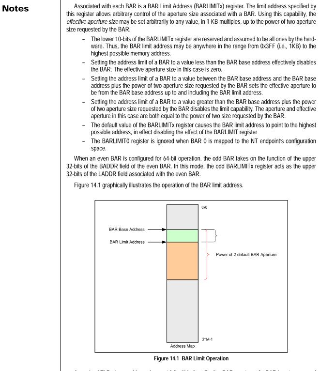
A received TLP whose address does not fall within the effective BAR aperture of a BAR is not processed by the BAR. A received TLP whose address falls within a BAR aperture, but outside the *effective BAR aperture*, is treated as an unsupported request by the NT function. The behavior for TLPs whose address falls within the effective address of multiple BARs is undefined.
