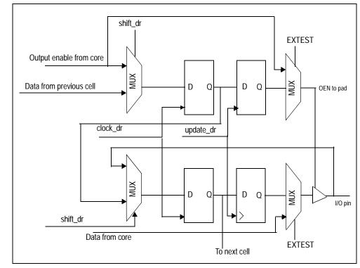
Figure 25.5 Diagram of Bidirectional Cell
