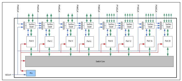
Figure 2.1 Logical Representation of PES32NT8AG2 Clocking Architecture
