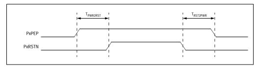
Figure 11.4 Power Enable Controlled Reset Output Mode Operation
