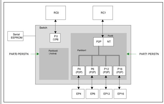
Figure 26.15 Active/Active System Configuration Before Failover Event
