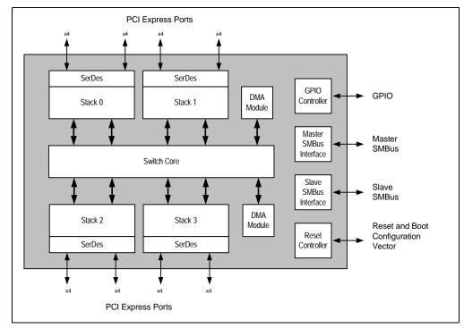
Figure 1.1 PES32NT8xG2 Block Diagram
