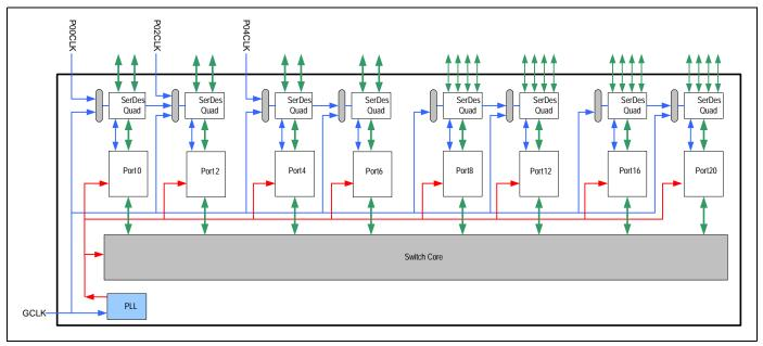
Figure 2.2 Logical Representation of PES32NT8BG2 Clocking Architecture
