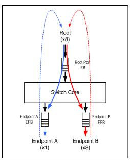
Figure 4.3 PCI Express Switch Static Rate Mismatch
