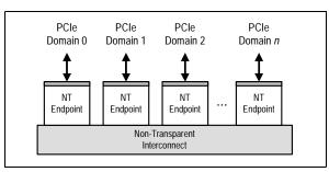
Figure 1.6 Generalized Multi-Port Non-Transparent Interconnect
