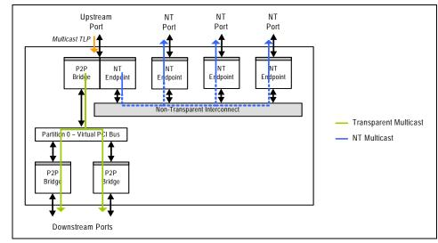
Figure 17.3 Transparent and Non-Transparent Multicast
