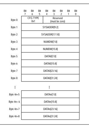
Figure 12.3 Sequential Double-word Initialization Sequence Format
