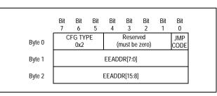
Figure 12.4 Jump Configuration Block
