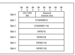
Figure 12.2 Single Double-word Initialization Sequence Format
