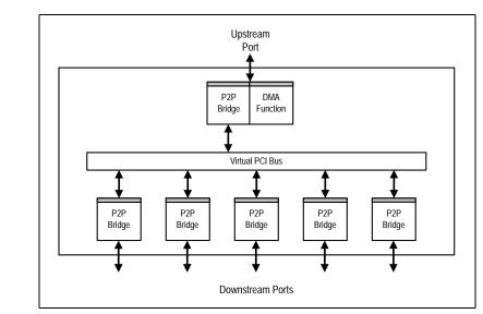
Figure 1.12 Switch Partition with DMA function
