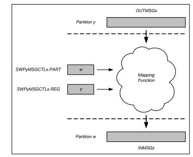
Figure 14.10 Logical Representation of Message Register Operation
