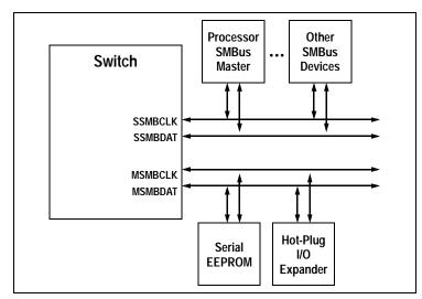
Figure 12.1 Split SMBus Interface Configuration
