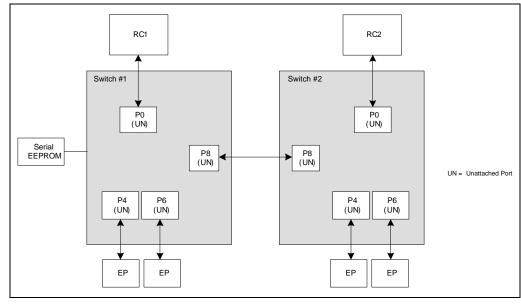
Figure 26.8 System Configuration immediately after Switch Fundamental Reset
