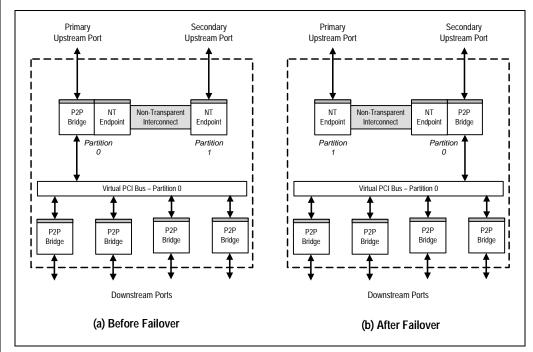
Figure 1.15 Non-Transparent Switch Failover Usage
