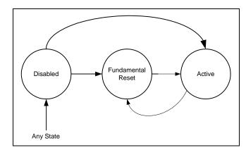
Figure 5.1 Allowable Partition State Transitions
