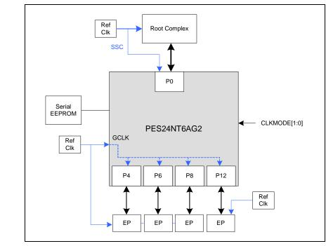
Figure 26.2 PES24NT6AG2 with Ports Operating in Different Clock Modes
