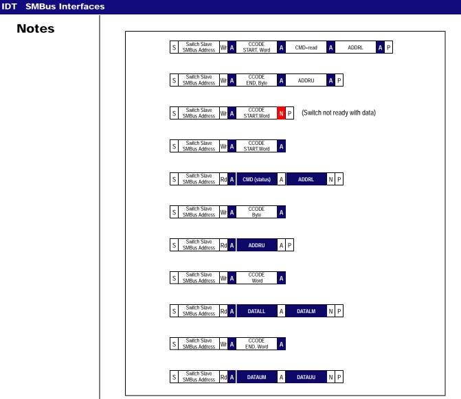
Figure 12.17 CSR Register Read Using SMBus Read and Write Transactions with PEC Disabled
