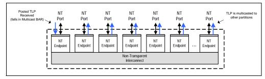
Figure 1.18 Example of Non Transparent Multicast
