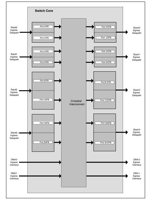
Figure 4.1 High Level Diagram of Switch Core
