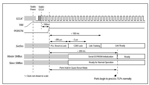
Figure 3.1 Switch Fundamental Reset with Serial EEPROM Initialization
