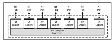
Figure 1.10 Non-Transparent Switch with Non-Transparent Ports
