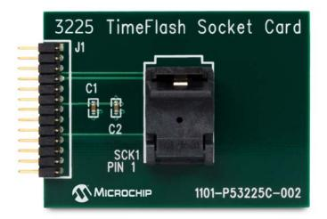
Single socket card,  $3.2 \times 2.5 \text{ mm}$  with 10 blank DSC8001 parts for TimeFlash Oscillator Programmer
