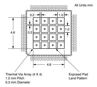
Figure 8. Recommended Solder Mask Openings
