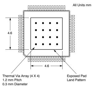
Figure 7. Recommended Thermal Land Pattern
