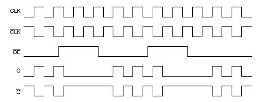
Figure 4. Output Enable (OE) Timing Diagram
