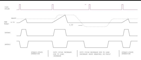
Figure 4 – PWM Operating Waveforms
