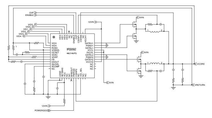
Figure 13. 12V Control, 5V Power, VR10.0 Converter
