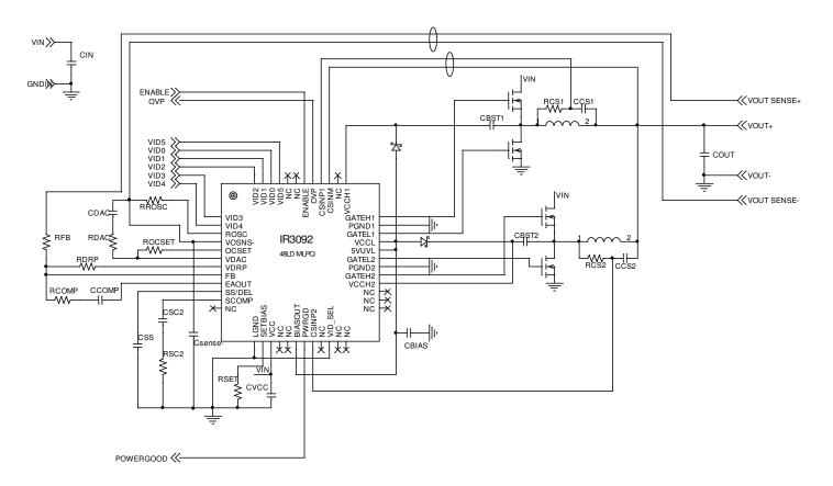
Figure 6 – System Diagram
