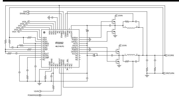
Figure 12. 12V Control, 12V Power Opteron Converter
