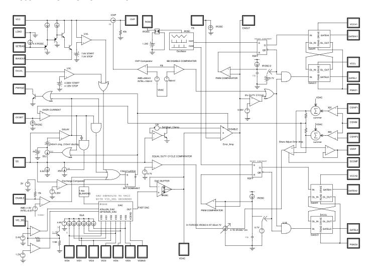
Figure 1 – IR3092 Block Diagram
