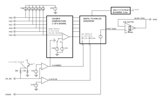
Figure 7- VID Control Block Diagram
