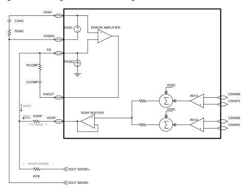
Figure 9 - Adaptive voltage positioning
