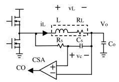
Figure 5 – Inductor Current Sensing and Current Sense Amplifier
