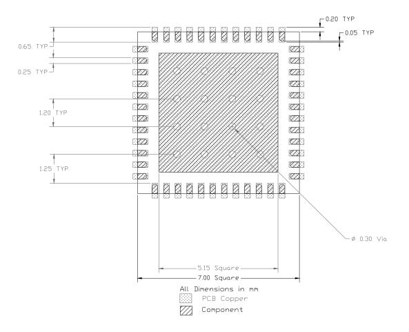
Figure 15. PCB metal and component placement.
