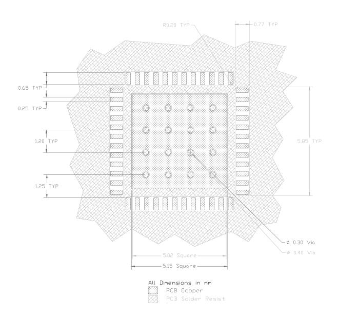
Figure 14. PCB metal and solder resist.
