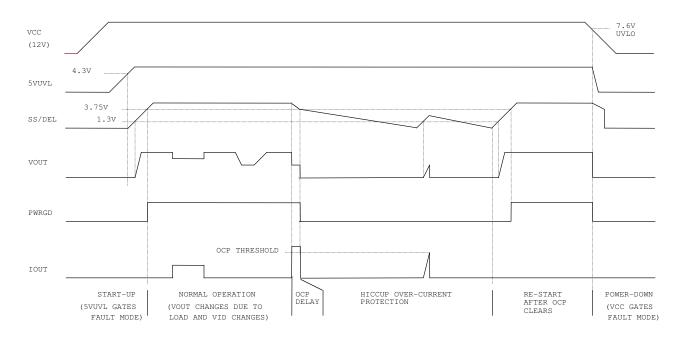
Figure 8 - Operating Waveforms
