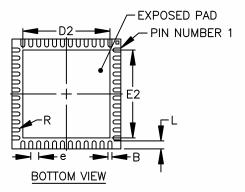
NOTE 1: DETAILS OF PIN #1 ARE OPTIONAL, BUT MUST BE LOCATED WITHIN THE ZONE INDICATED. THE IDENTIFIER MAY BE MOLDED OR MARKED FEATURES.
