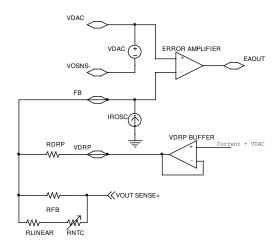
Figure 10- Temperature compensation of inductor DCR
