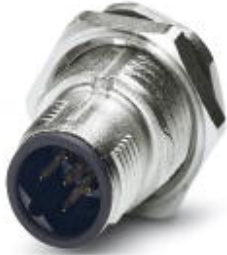
Sensor/actuator flush-type connector, 5-pos., M12 SPEEDCON, B-coded, rear/screw mounting with Pg9 thread, with straight solder connection
