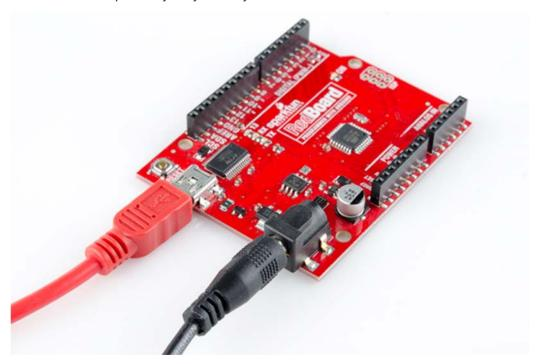
It is acceptable to connect both a barrel jack and a USB connector at the same time. The RedBoard has power-control circuitry to automatically select the best power source.
