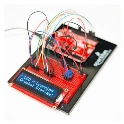
For more ideas, check out the SparkFun Inventor's Kit, which centers around the RedBoard, and teaches you how to connect it up to buttons, relays, flex sensors, and other components.
