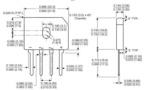
Polarity shown on front side of case, positive lead by beveled corner
