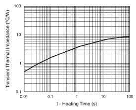
Fig. 6 - Typical Transient Thermal Impedance
