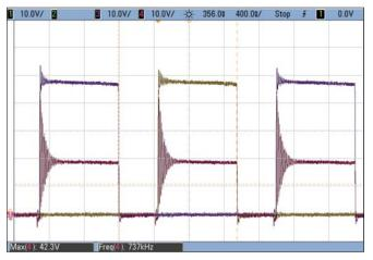
Figure 4: Typical waveforms taken at 48  $V_{\rm IN}$  to 12  $V_{\rm OUT}/15$   $A_{\rm OUT}$  CH1: Primary side switch node A voltage - CH3: Primary side switch node B voltage - CH4: Secondary side bridge voltage
