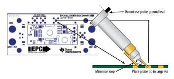
Figure 3: Proper Measurement of Switch Nodes or Output Voltage
