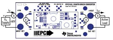
Figure 2: Proper Connection and Measurement Setup
