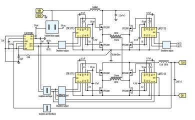
Figure 1: Block Diagram of EPC9102 Demonstration Board
