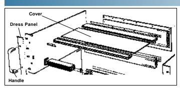
Panels provide maximum protection for card cage interiors. Perforated to insure proper airflow. Constructed from .062" aluminum, satin finish with clear irridite plating. Covers slide into T-strut grooves, no mounting hardware required.
