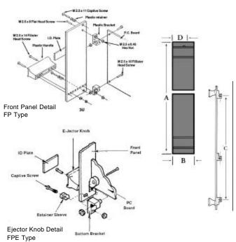
Screw mounted front panel kit include handle and identification panel. Available in 3U, 6U, and 9U heights and in two widths: 4HP (0.778") and 8HP (1.588"). All mounting hardware, including board mounting support bracket and hardware also included. Panel with clear chromate plating matches standard finish for Vector packaging products.
