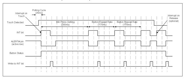
FIGURE 5-3: Sensor Interrupt Behavior - No Repeat Rate Enabled
