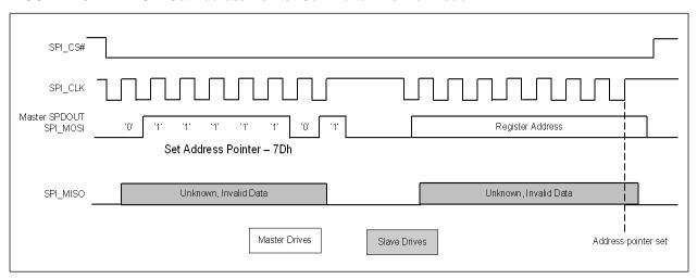
FIGURE 4-5: SPI Set Address Pointer Command - Normal Mode
