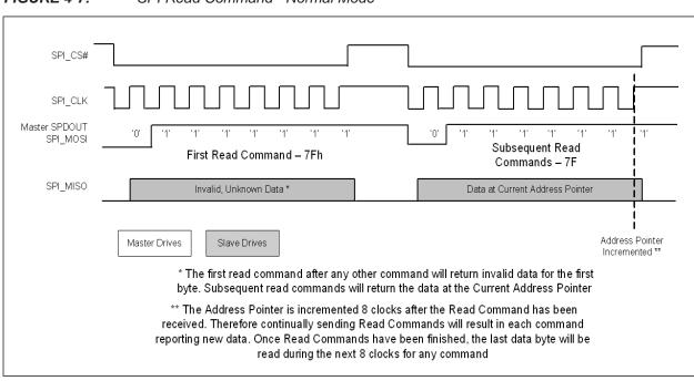
FIGURE 4-7: SPI Read Command - Normal Mode
