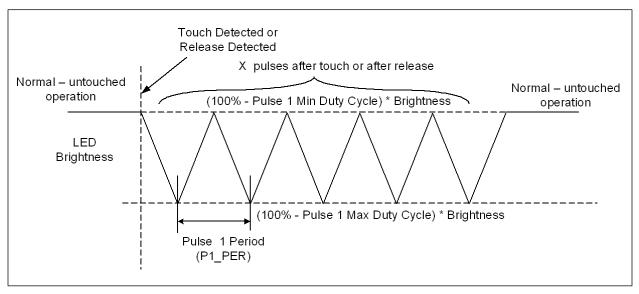
FIGURE 6-2: Pulse 1 Behavior with Inverted Polarity
