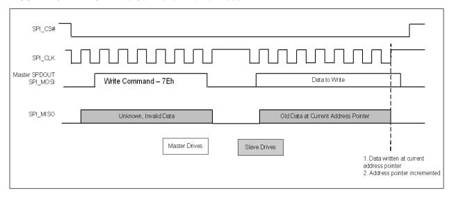
FIGURE 4-6: SPI Write Command - Normal Mode
