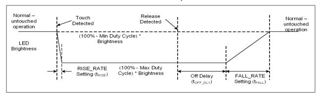
FIGURE 6-8: Direct Behavior for Inverted Polarity
