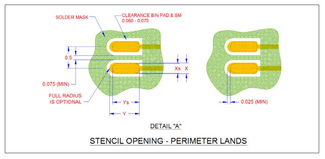
FIGURE 7-5: CAP1188 PCB Detail B - 24-Pin QFN 4mm x 4mm
