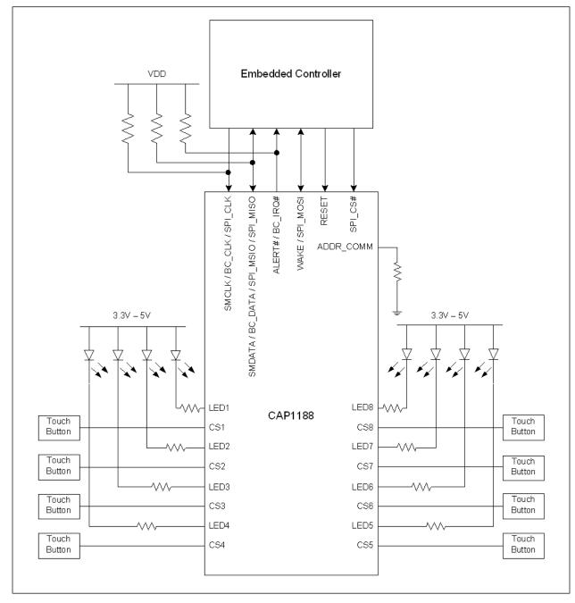
FIGURE 5-1: System Diagram for CAP1188
