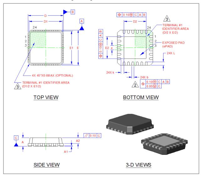
FIGURE 7-2: CAP1188 Package Dimensions - 24-Pin QFN 4mm x 4mm
