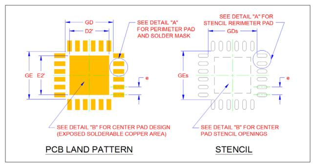
FIGURE 7-4: CAP1188 PCB Detail A - 24-Pin QFN 4mm x 4mm
