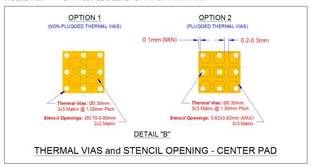
FIGURE 7-6: CAP1188 Land Dimensions - 24-Pin QFN 4mm x 4mm
