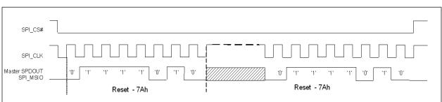
FIGURE 4-9: SPI Reset Interface Command - Bi-directional Mode
