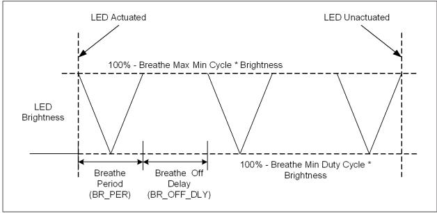
FIGURE 6-6: Breathe Behavior with Inverted Polarity
