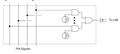
While the routing delays of channel-based routing schemes in masked or FPGAs are cumulative, variable, and path-dependent, the MAX 7000 PIA has a fixed delay. The PIA thus eliminates skew between signals and makes timing performance easy to predict.
