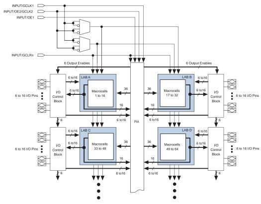
Figure 2 shows the architecture of MAX 7000E and MAX 7000S devices.
