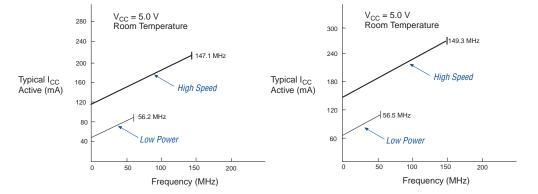
Figure 15. I<sub>CC</sub> vs. Frequency for MAX 7000S Devices (Part 2 of 2)
