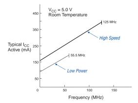
Figure 14. I<sub>CC</sub> vs. Frequency for MAX 7000 Devices (Part 2 of 2)
