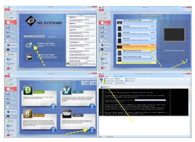
In the 'Tools' menu of the Serial Environment, is a button called 'SPE Load'. SPE stands for "Serial Platform Environment". If your display module is connected to the PC via the 4D Systems Programming Cable, clicking this button will load a special 4DGL application onto your module. This application is known as the SPE Application, and will enable your chosen module to run as a Serial Slave.
