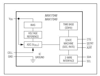
Figure 2. Block Diagram
