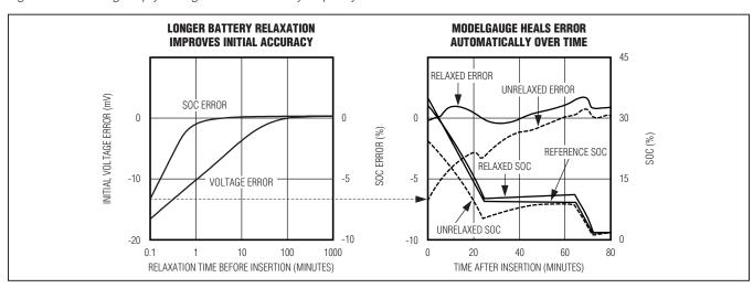
Figure 5. ModelGauge Heals Error Automatically
