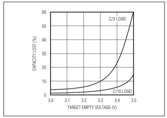
Figure 4. Increasing Empty Voltage Reduces Battery Capacity
