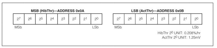
Figure 9. HIBRT Register Format
