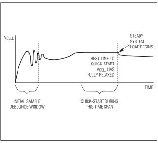
Figure 7. Insertion Waveform Requiring Quick-Start Command
