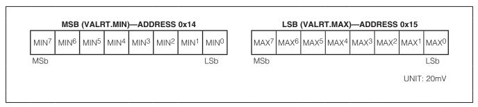
Figure 11. VALRT Register Format
