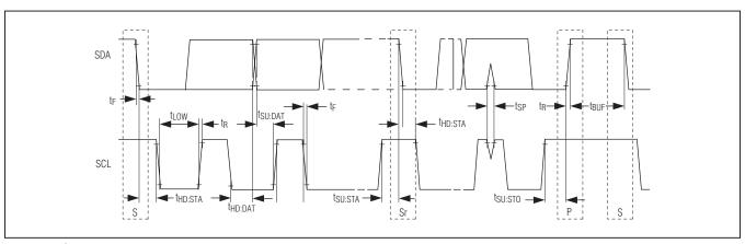
Figure 1. I2C Bus Timing Diagram
