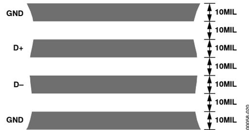
Figure 20. Arrangement of Signal Tracks
