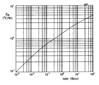
Fig 2. Transient thermal impedance characteristic per leg
