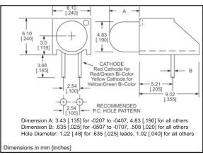
Standard Polarity shown in drawing: Cathode right
