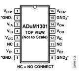
\*PIN 2 AND PIN 8 ARE INTERNALLY CONNECTED, AND CONNECTING BOTH TO GND, IS RECOMMENDED. PIN 9 AND PIN 15 ARE INTERNALLY CONNECTED, AND CONNECTING BOTH TO GND<sub>2</sub> IS RECOMMENDED.
