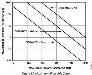
Figure 17. Maximum Allowable Current for Various Current-to-ADuM1300/ADuM1301 Spacings
