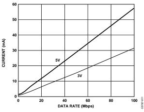
Figure 9. Typical ADuM1300 V<sub>DD1</sub> Supply Current vs. Data Rate for 5 V and 3 V Operation
