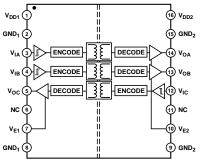
Figure 2. ADuM1301 Functional Block Diagram
