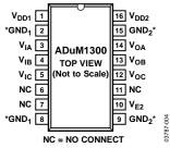
\*PIN 2 AND PIN 8 ARE INTERNALLY CONNECTED, AND CONNECTING BOTH TO GND1 IS RECOMMENDED. PIN 9 AND PIN 15 ARE INTERNALLY CONNECTED, AND CONNECTING BOTH TO GND<sub>2</sub> IS RECOMMENDED.
