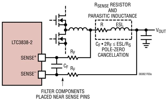
Figure 3a. R<sub>SENSE</sub> Current Sensing
