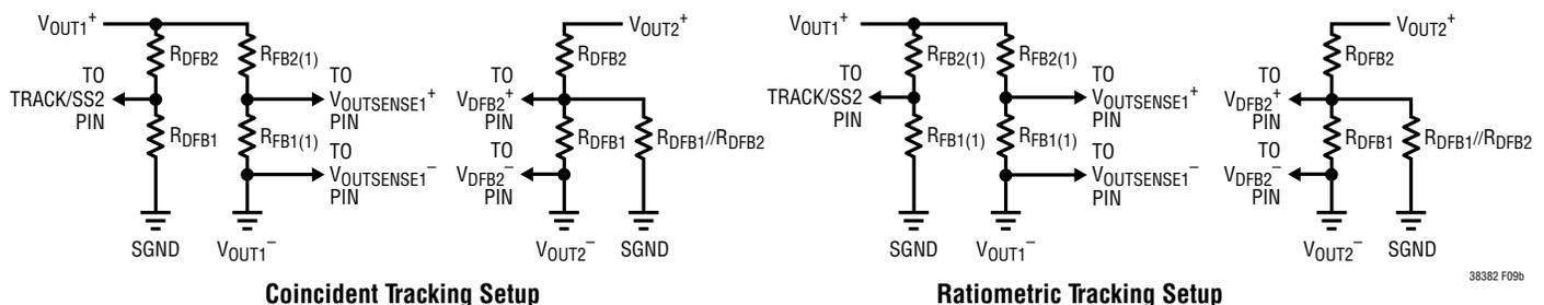
Figure 9b. Setup for Coincident and Ratiometric Tracking
