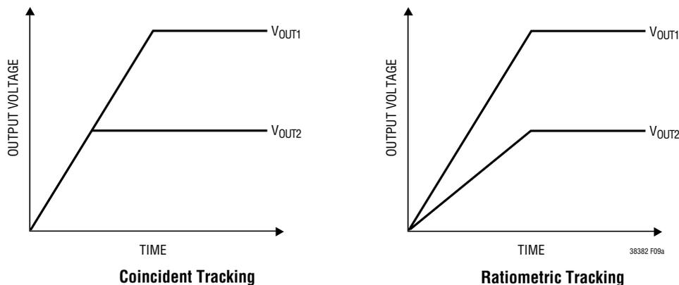
Figure 9a. Two Different Modes of Output Tracking
