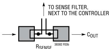
Figure 3b. Sense Lines Placement with Sense Resistor
