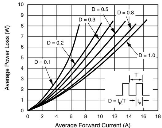
Fig. 2 - Forward Power Dissipation Characteristics Per Diode
