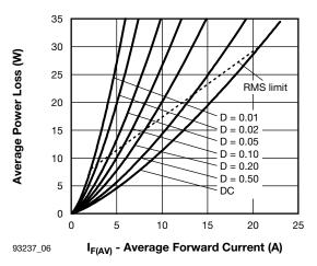
Fig. 6 - Forward Power Loss Characteristics
