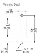
Panel Mounting Detail Tolerance ±.005 [.13] unless noted.
