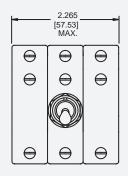
Panel Mounting Details: Tolerance ±.005 [.13] Unless noted.
