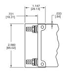
NOTE: THIS BARRIER CAN BE FLIPPED TO COVER EITHER POLE. PLEASE CONTACT FACTORY FOR SPECIFIC PART NUMBER
