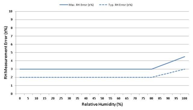
Figure 2. RH Accuracy at 30 °C
