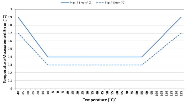
Figure 3. Temperature Accuracy\*
