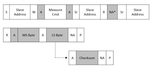
\*Note: Device will NACK the slave address byte until conversion is complete.
