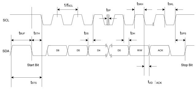
Figure 1. I<sup>2</sup>C Interface Timing Diagram
