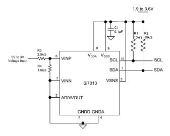
Figure 7. Typical Application Circuit for Single Ended 0 to 3 V Measurement
