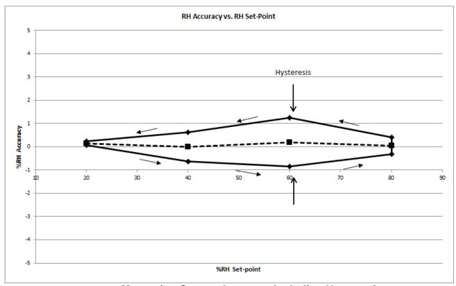
Figure 9. Measuring Sensor Accuracy Including Hysteresis
