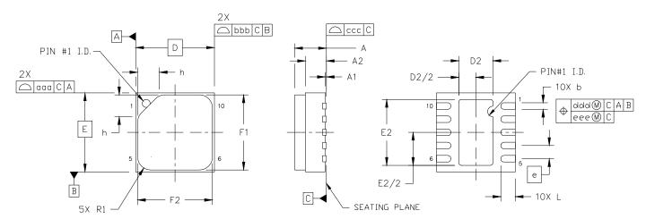
Figure 12. 10-pin DFN with Protective Cover
