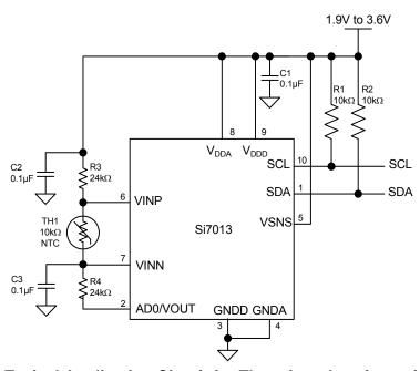
Figure 5. Typical Application Circuit for Thermistor Interface with AD0 = 1
