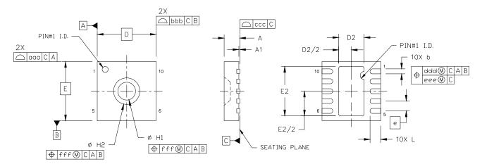
Figure 11. 10-pin DFN Package Drawing
