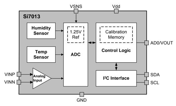
Figure 8. Si7013 Block Diagram
