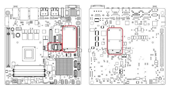
The AIMB-226 provides 1 Full size Mini PCI express slot to support mSATA (MINIPCIE1) and 1 Full size Mini PCI express slot to support SIM card holder (MINIPCIE2).
