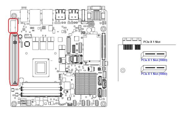
AIMB-226 provides 1x PCI express x16 slot and 1x golden-finger PCIex1
