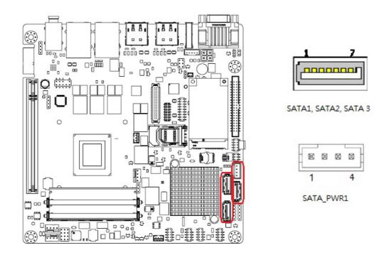
AIMB-226 features a high performance Serial ATA interface (up to 600 MB/s) which eases cabling to hard drives with long, thin cables.
