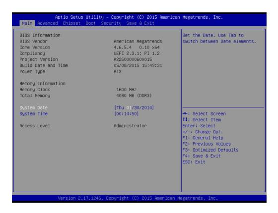
The Main BIOS setup screen has two main frames. The left frame displays all the options that can be configured. Grayed-out options cannot be configured; options in blue can. The right frame displays the key legend.
