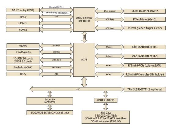
Figure 1.2 AIMB-226 Board Diagram
