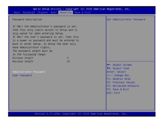
Select Security Setup from the AIMB-226 Setup main BIOS setup menu. All Security Setup options, such as password protection and virus protection, are described in this section. To access the sub menu for the following items, select the item and press <Enter>: Change Administrator / User Password.
