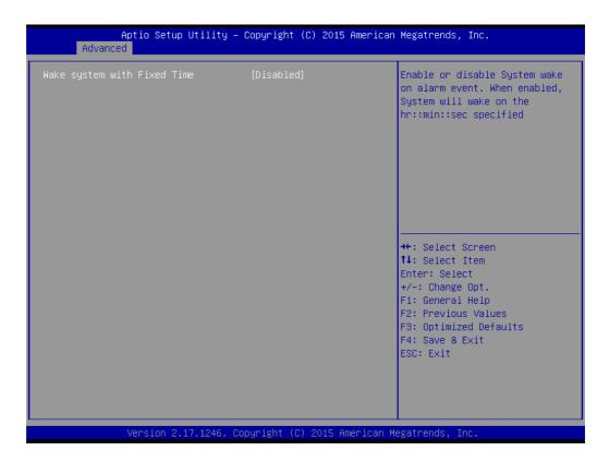
Wake system with fixed time Enable or disable system wake on alarm event.
