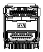
The AIMB-226 includes two DP++, which can support DP outputs and convert to HDMI through DP-to-HDMI cables. Pin assignments for DP++ and HDMI are detailed in Appendix B.
