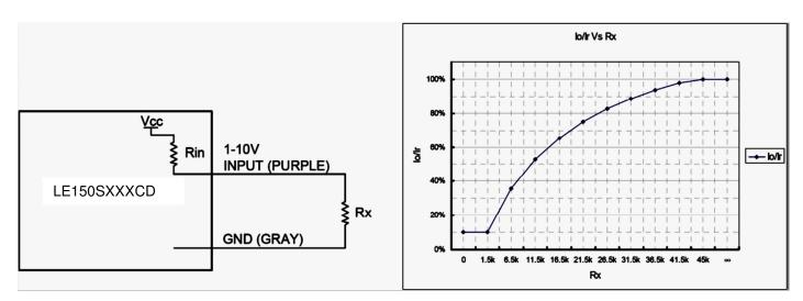
**Dimming Configuration using External Resistance**
