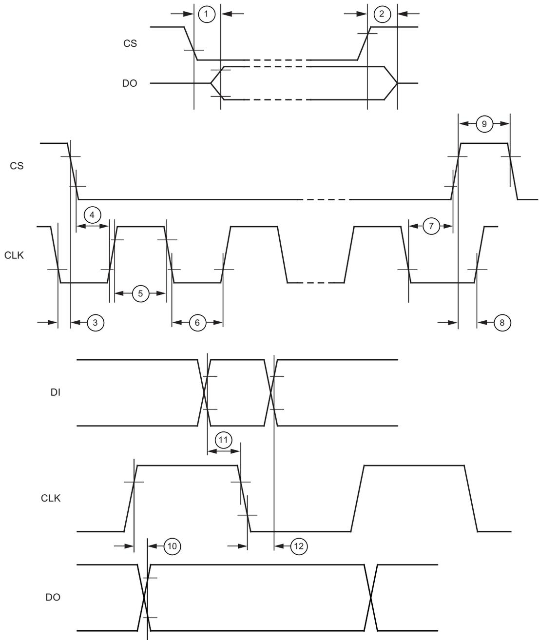
Inputs DI, CLK, CS: High level =  $0.7 \times V_{CC}$ , low level =  $0.3 \times V_{CC}$
