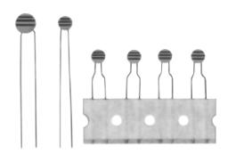
Disc type negative temperaturecoefficient thermistors. Resistance values from 8  $\Omega$  to 150  $k\Omega$  and B Values are from 3000 K to5000 K.
