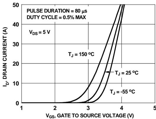
Figure 5. Transfer Characteristics
