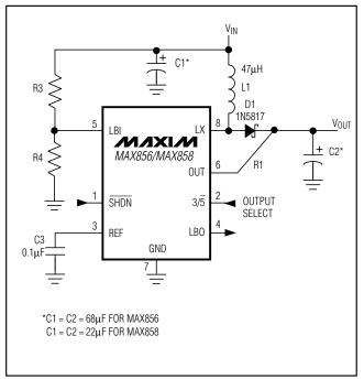
Figure 2a. Standard Application Circuit—Preset Output Voltage
