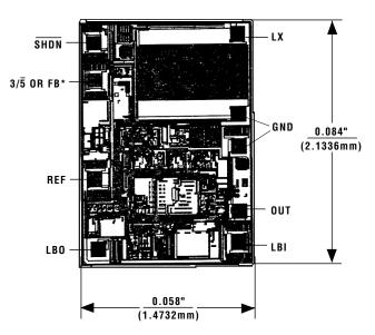
$*3/\overline{5}$  FOR MAX856/MAX858; FB FOR MAX857/MAX859. TRANSISTOR COUNT: 357; SUBSTRATE CONNECTED TO OUT.
