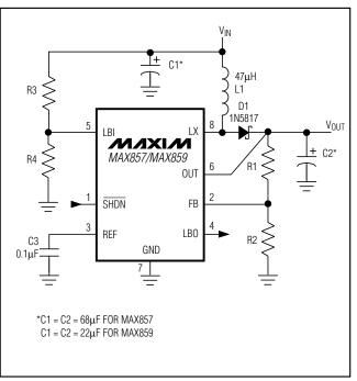
Figure 2b. Standard Application Circuit—Adjustable Output Voltage
