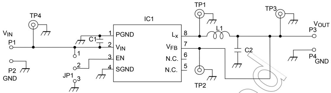
**Figure 6 Circuit of the Board Layout Example**
