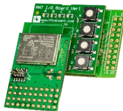
Figure 3-2. D52Q Module stacked on IO and Battery Boards.
