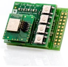
Figure 3-1. N5 Module stacked on IO and Battery Boards.
