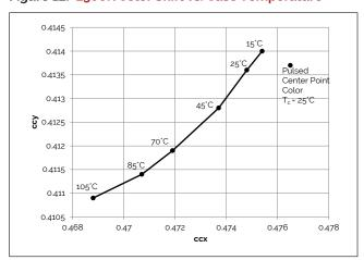
Figure 13: 2700K, 97 CRI Color Shift vs. Case Temperature<sup>1</sup>
