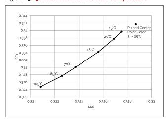
Figure 16: 3000K Class A Color Shift vs. Case Temperature<sup>1</sup>
