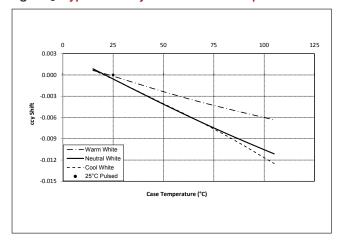
Figure 10: Typical DC ccx Shift vs. Case Temperature
