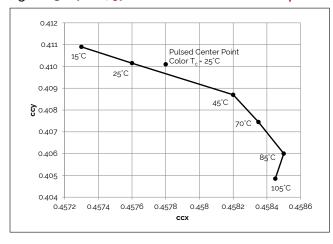
Figure 14: 3000K, 97 CRI Color Shift vs. Case Temperature<sup>1</sup>
