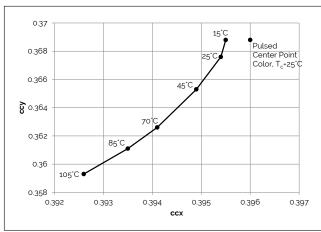
Figure 18: 4000K Class A Color Shift vs. Case Temperature<sup>1</sup>
