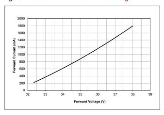
Figure 3: Vero SE 18D Drive Current vs. Voltage
