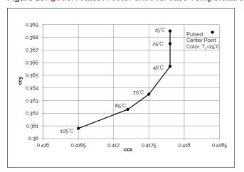
Figure 17: 3500K Class A Color Shift vs. Case Temperature<sup>1</sup>
