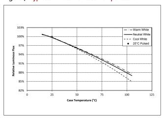
Figure 8: Décor Series Typical DC Flux vs. Case Temperature<sup>4</sup>
