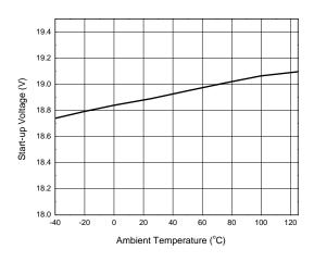
Minimal Operating Voltage vs. Ambient Temperature
