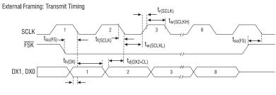
NOTES: Data valid on transmit outputs until SCLK rises. The most significant bit is shifted first.
