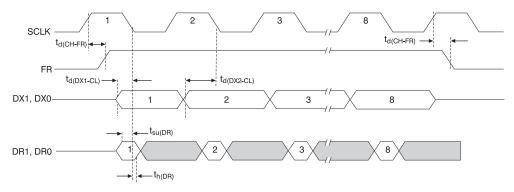
Note: The most significant bit is shifted first.
