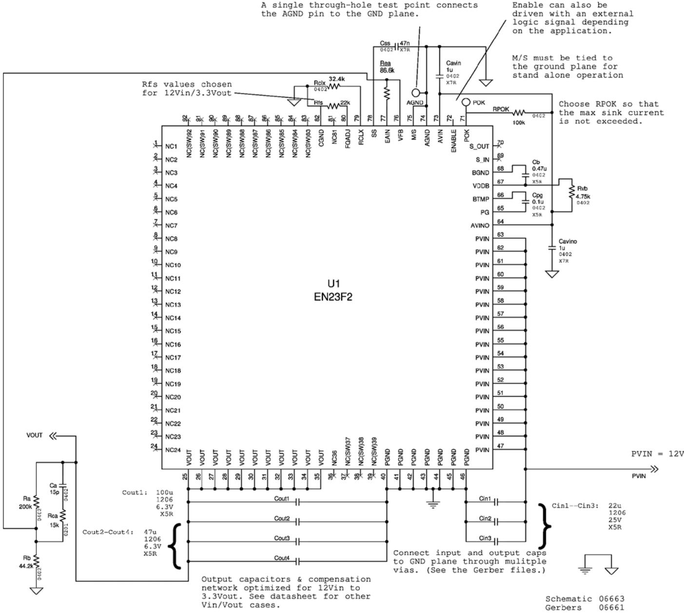
Figure 13: Engineering Schematic
