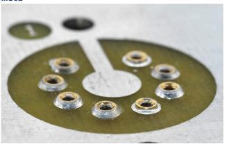
Part number MS02 consists of a package of 8 cage jacks. These are mounted directly in a print circuit board. Use a spacer between the PCB and the heatsink to avoid short circuits.
