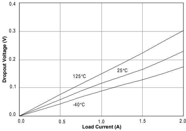
Dropout Voltage at  $V_o = 1.5V$
