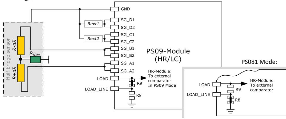
An alternative way of connecting a half bridge to PS09 is shown below, where the unused ports C and D are connected parallel to Ports A and B respectively. The external resistors are avoided in this connection. The option for using an external comparator is available only on the HR-module.
