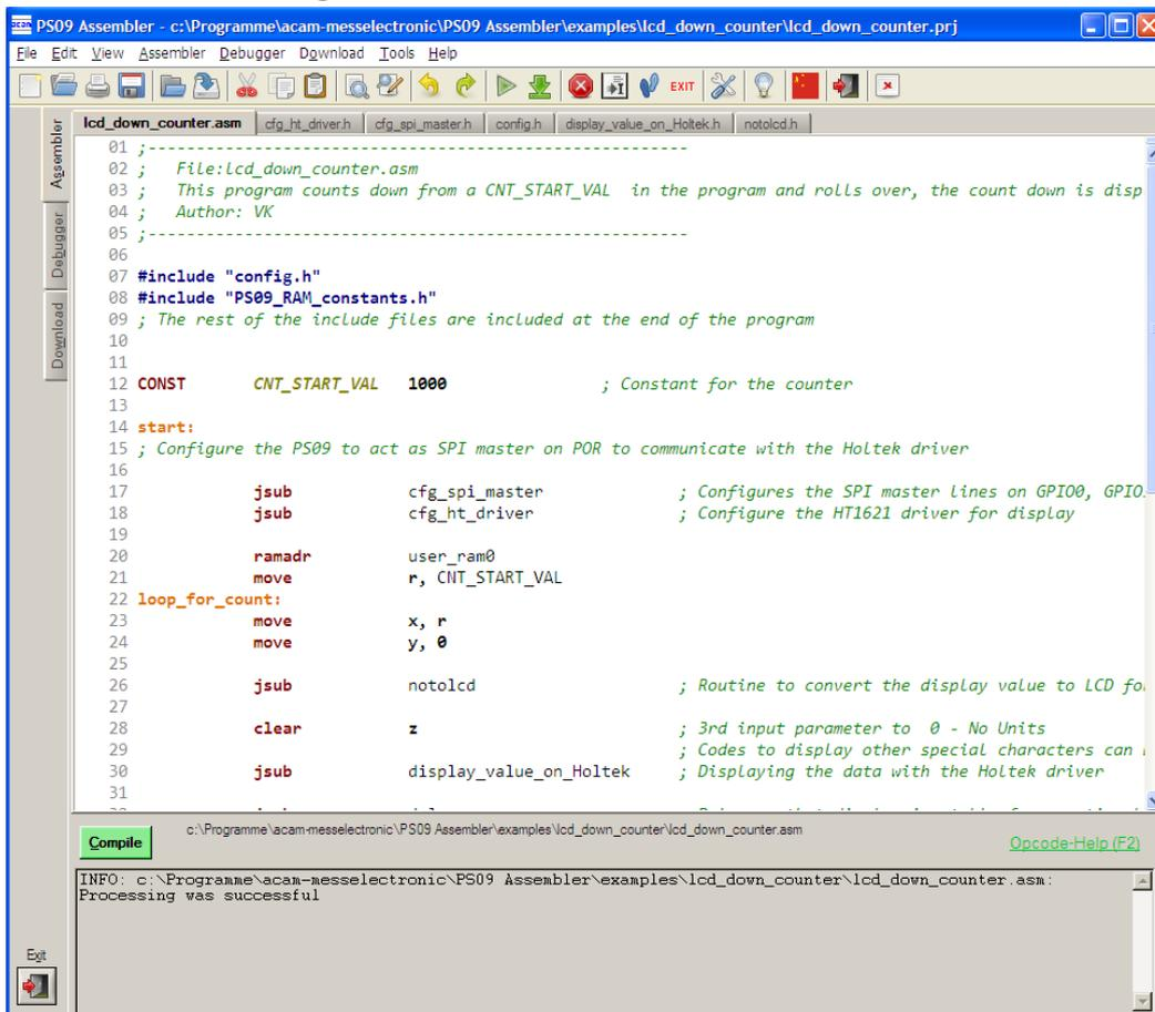
The 'Assembler' tab page is the main window to open all the source code and include files. It consists of a status message window at the bottom and buttons to operate the assembler. By clicking the green link labeled ,Opcode-Help [F2]'an integrated online help pops up which provides detailed information about the available op codes.
