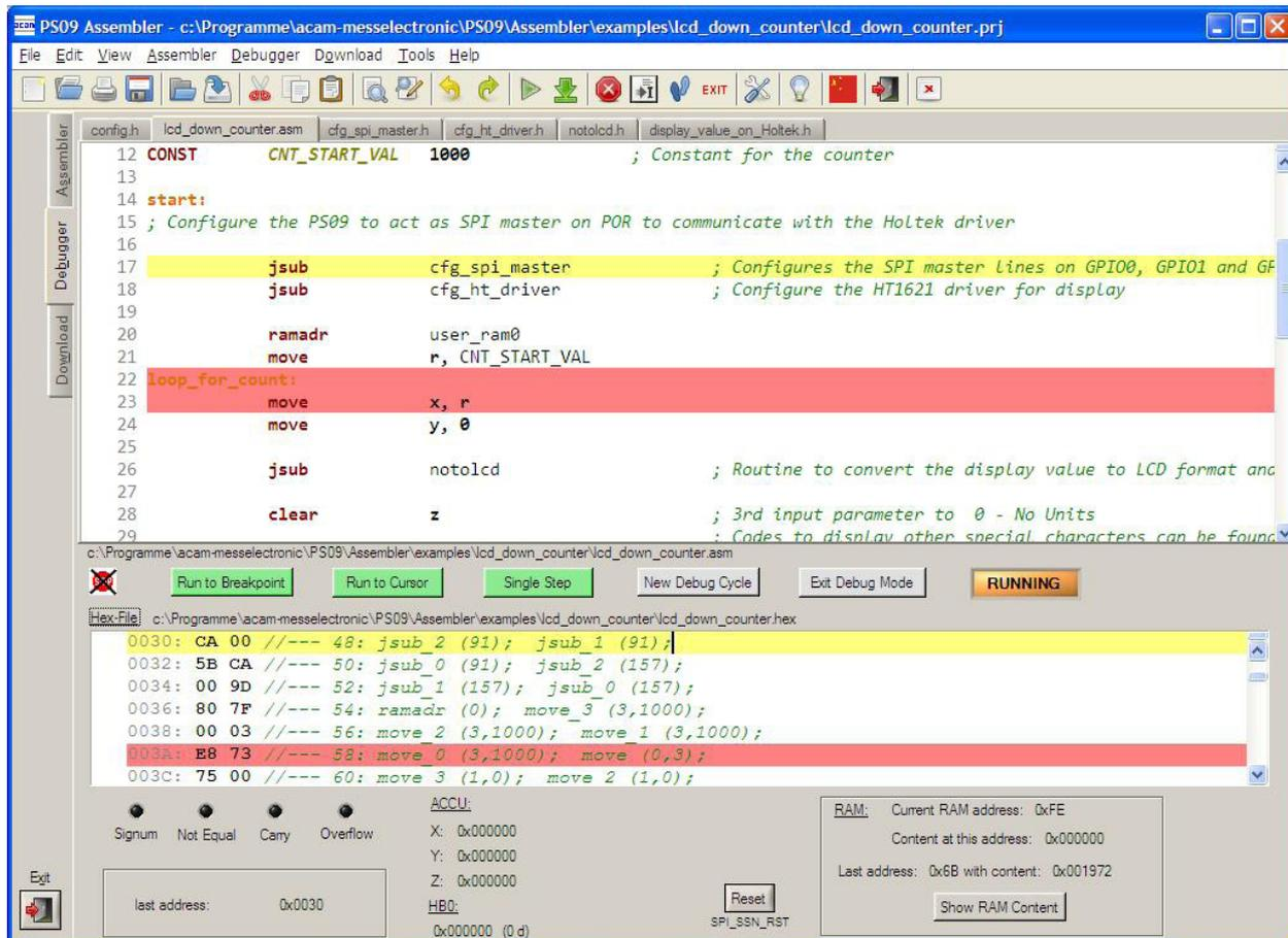
This tab provides a powerful debug interface. On this page you can debug the programs you wrote and make the processing of the code transparent. There are many data additionally available, e.g. status of the flags, content of the accumulator registers x,y,z or the content of the RAM. It is also possible to emulate the reset button. An active debugging process is indicated by a LED. There are several debug-modes available.
