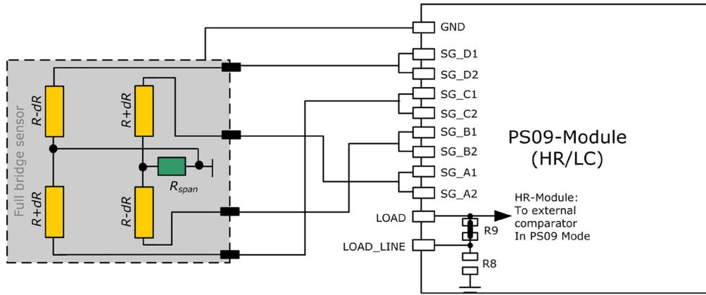
Existing sensors with Wheatstone bridge connection might be adapted just by changing the wiring according to the following picture.
