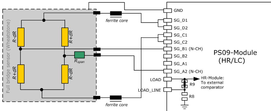
The PICOSTRAIN measurement principle is based on measuring the discharge time of a capacitor. For this reason the correct size and material of the capacitors is significant to achieve best measuring results. For Wheatstone, the discharging time is furthermore reduced by the factor of 0.7, The following formula can be used to calculate the discharging capacitance.
