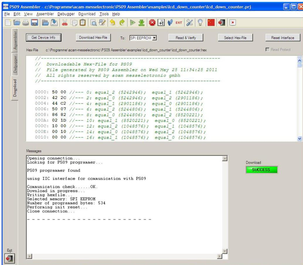
The 'Download' tab provides an interface to program the PS09 with the compiled hex code. For this purpose the hex-file is displayed and several buttons are provided to handle the download. A big message window shows the status of the connection and the programming. Furthermore a LED indicates success or failure of the download.
