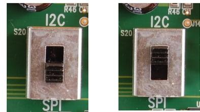
Figure 5-2: Switch IIC/SPI
