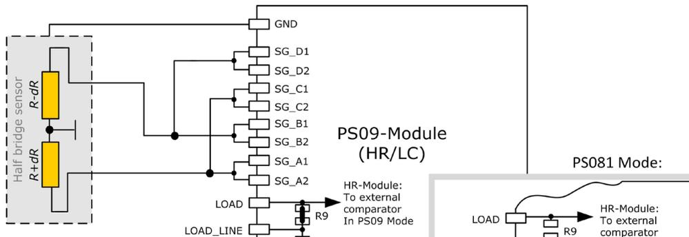
Please note: Both wiring options shown in figure 3a and 3b have to be done externally, i.e. at the solder pad of the module. There are no wiring or placement options on the module itself.
