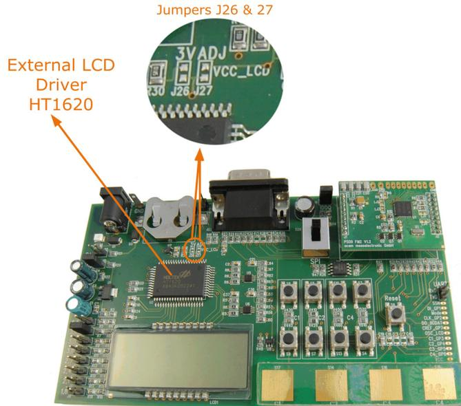
The following picture shows the connection of an external LCD driver circuit:
