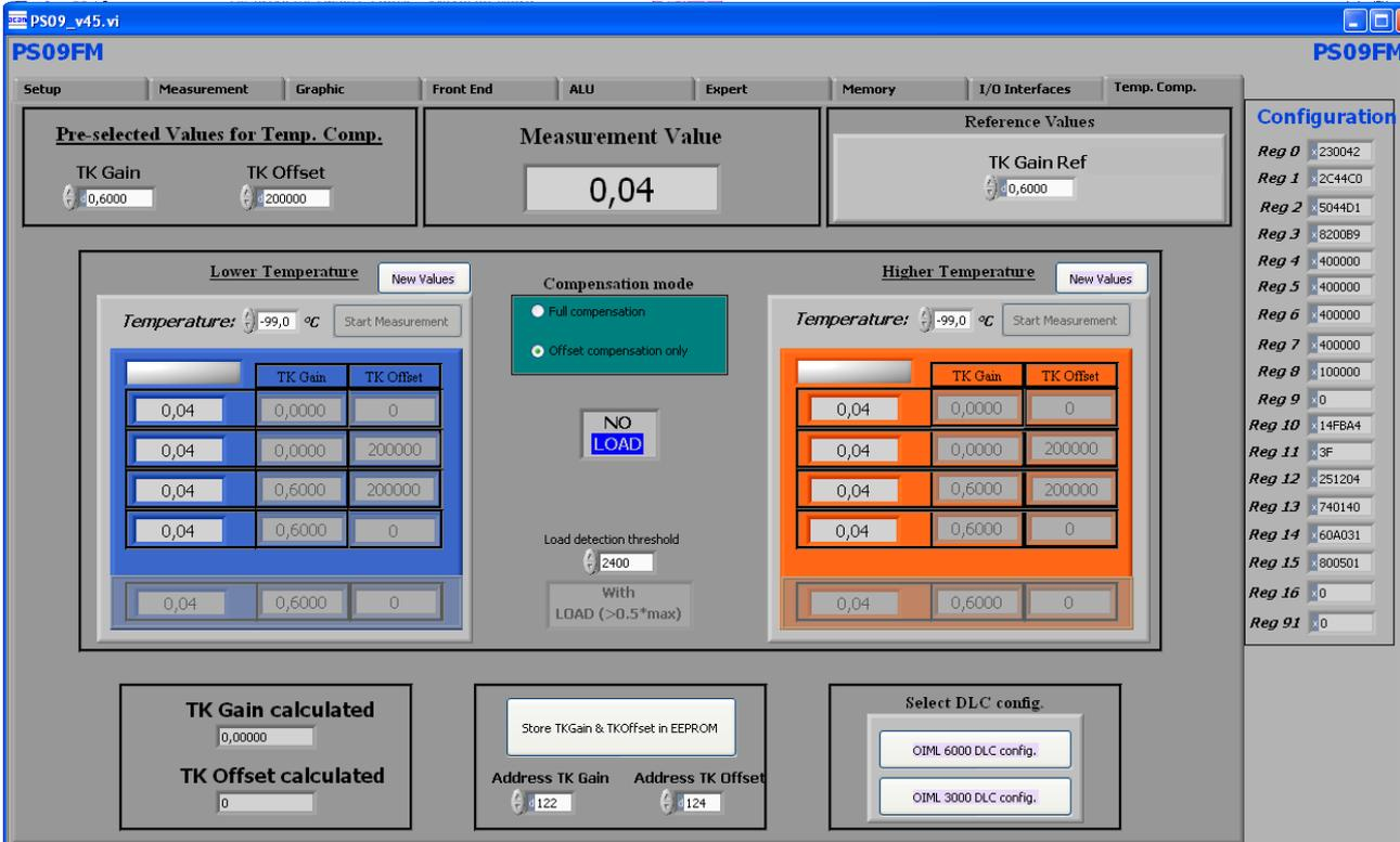
This page contains all the settings that are used for temperature compensation of a load cell system connected to the PS09. Either full compensation can be performed or only Offset compensation can also be done.
