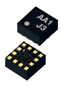
operating characteristics over the range of input supply voltages and virtually undetectable ratiometric error. The I<sup>2</sup>C digital protocol is used to communicate with the chip to configure the part and monitor outputs.
