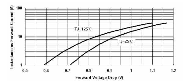
Fig.3-Typical Instantaneous Forward Voltage Characteristics
