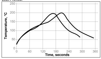
High air flow rates give as even a temperature distribution as possible. However, across the board, this may contribute to exhaustion of paste activity. LOCTITE WS 200 combines excellent printing characteristics with tolerance of hot profiles and high air flow rates, although extreme (long & hot) profiles may still give sub-optimal reflow and cleaning in some oven types.
